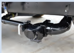
Pivoting Sewer Head for Easy Positioning and Better Ground Clearance
